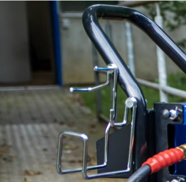
Fig. 33: Hanger for storing the lance
