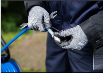
Fig. 26: Screwing on the pipe cleaning nozzle
