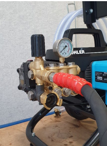
Fig. 34: Connecting hose plugged in
