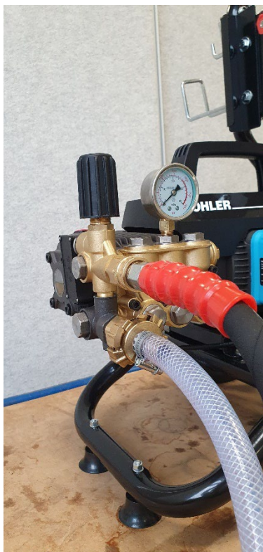
Fig. 23: Connection to the water supply marked with transparent hose
