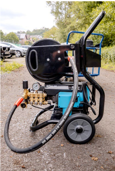
Fig. 22: Connecting the black connecting hose
