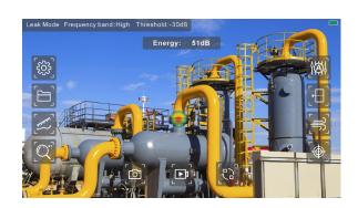
The camera supports real-time monitoring of audio signals via Bluetooth connection to headphones. It also supports the online display of frequency spectrum diagrams.
