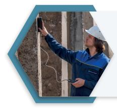
Concrete Cover Meter NOVOTEST Rebar Detector is used to measure the thickness of the concrete cover, determine the location and estimate the diameter of rebar in reinforced concrete products in the conditions of enterprises, construction sites, buildings and structures in use.
