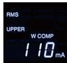
▲AC Hipot (Withstanding voltage) test settings display (example)
