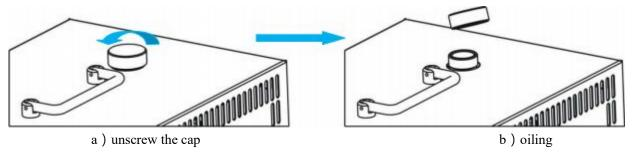
Note: The oil filling level is between the Min and Max scales of the display window
