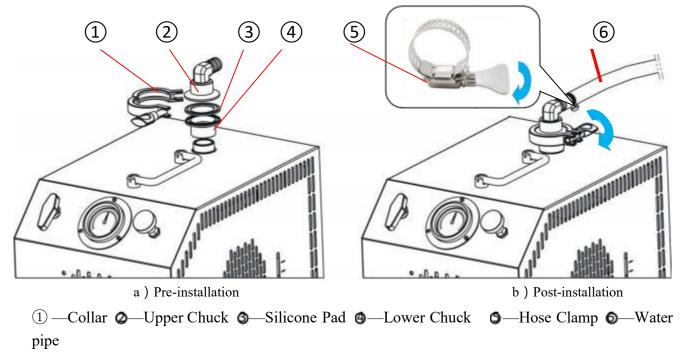
Note: 1. the inner diameter of the water pipe is 19mm. The user can purchase it according to the actual length for use, with moderate hardness, which is convenient for clamping and ensures a smooth aerosol channel.
